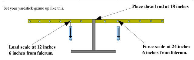
While holding down on the load scale, pull down on the force scale. Never allow either scale to
