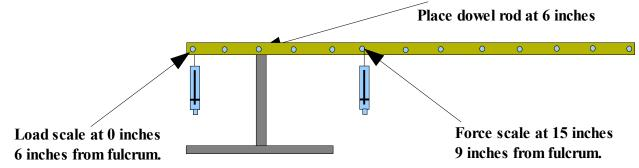
While holding down on the load scale, pull down on the force scale. Never allow either scale to
